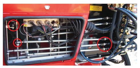
All ball joints must be lubricated monthly. Do not forget the ball joints on the spool ends. The image shows examples of the location of the ball joints.
