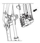
4. **Cranes with S-boom:** Extend the boom extensions until the catcher ② drops. Retract the extensions carefully until the catcher secures the boom. Start to lower the first boom until the second boom is in horizontal position.
