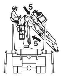
5. Retract the extensions until it is locked by the catch. Slowly operate the 1st boom against the column.
