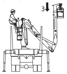
3. Retract the hydraulic extensions until the grapple is locked in the support.
