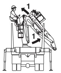
1. Drive the extensions out until it is released from the catch. Then, operate the 1st boom 1-1,5m out from the column.
