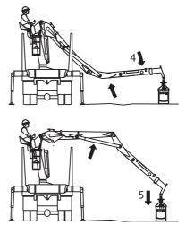
4. Press the grapple against the ground and straighten the 2nd boom.
