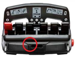
It is easy to switch between CTC and normal crane mode by pressing a button on HIAB's hand controller XSDrive (top) or CombiDrive (bottom).
