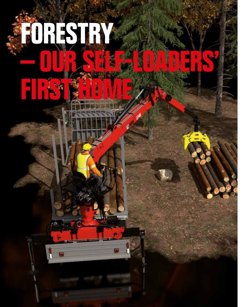
Our new self-loaders are in their element in the forest and suitable for a variety of tasks. Choose between two capacities and be sure to get the right machine for the job. The HIAB J14S is ideal for cut-to-length logging while our larger HIAB J24S, comfortably handles tree length logging. Both models deliver the industry's leading capacity to weight ratio.
