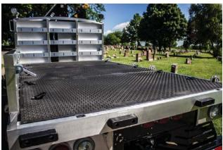
Fold down racking allows for easy side loading and unloading. Built with only 1/4" gap at the bottom of the gate to keep your supplies secured while driving. Rear flush design is dock ready. Contact your Hiab representative to start utilizing your one man operation.
