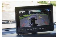
The monument series truck has 3 cameras that allow for a 180 degree view of the rear and sides of the truck. This combined with the cab-over design, nimble maneuverability, and a narrow truck bed allow for even easier navigations through the toughest of spots.
