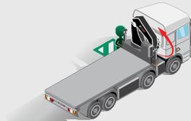
1. If the stabiliser system is manually controlled, push button
