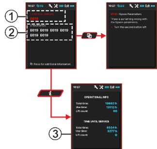
The different information shown in the alternative VIEWS depends on the crane configuration. Push the button to change between the different alternative displays for the INFO VIEWS and get extra information.
