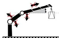
If the 2nd boom is down, the following movements are locked:
