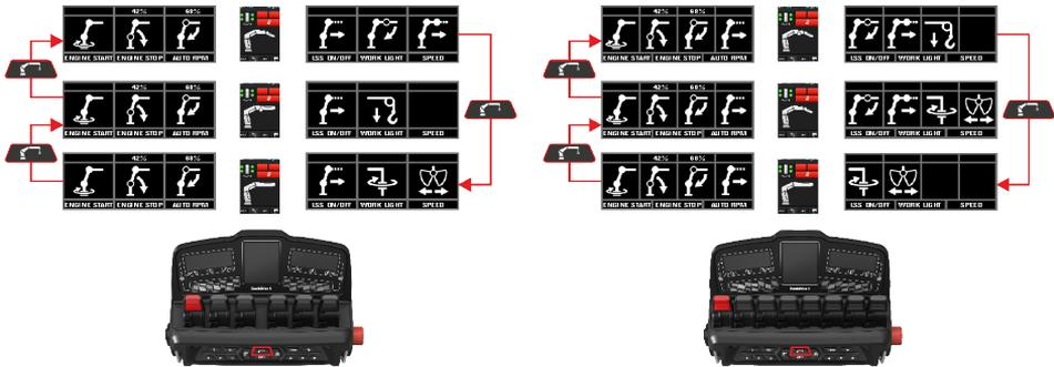
When the operator pulls out the emergency stop button on the controller, it always starts in CRANE 1 VIEW. The sub-VIEWS in CRANE VIEW are configured in production but can be changed by Effer service personnel.
