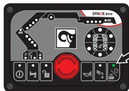
2. If using remote control, the crane will start in remote mode automatically. Push button (1) on the controller to change between the different crane menus or CRANE VIEWS.
