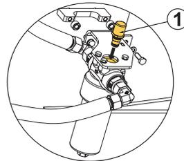
The return oil filter is on the oil tank, and can have a clogging indicator. This indicator turns red when needed. In all other cases (if the filter time is expired or without clogging indicator), you must follow the general recommendations for its replacement.
