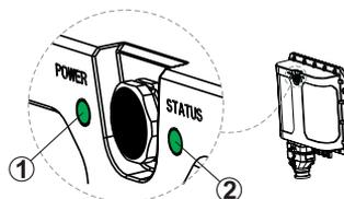
The LED is steady green = the gateway is operational and all connections are correct.
