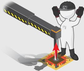
The procedure of operating the stabiliser legs can differ depending on the type of stabiliser leg. Repeat the instructions for the stabiliser extension and leg on the other side of the vehicle. For auxiliary stabiliser system [option]: Repeat the process.
