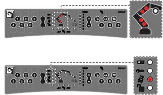
**Stabiliser system OLP:** No indication on the controller. See indications on the User Interface.
