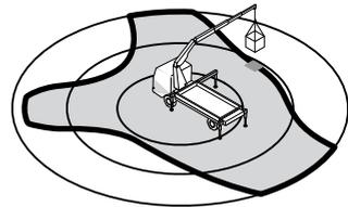
The position of both, **crane stabiliser extensions** and **auxiliary stabiliser extensions**, are detected proportionally by Progress to calculate the stability.
