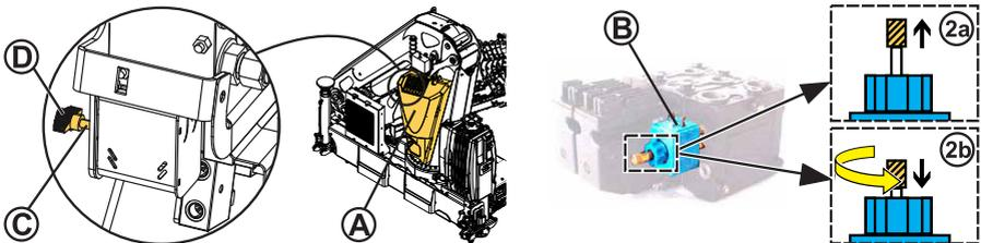
3. The shaft (C) may be provided with a knob (D) or with a hexagonal head screw.
