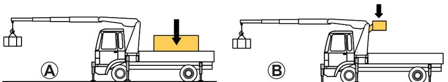
To tell Progress that you are using a ballast/counterweight, activate the detection with the related selector. When the system recognises correctly the ballast/counterweight, you will hear a double beep sound.
