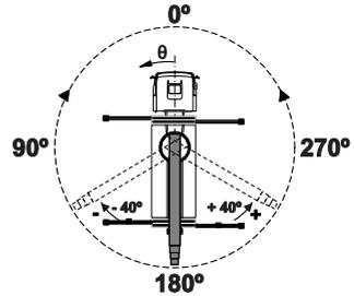
180°). Use the rotary selector (14) in the STEADY and the arrow keys in SCANRECO to change this value increasing or decreasing 10° at a time. The values of the simulation will be automatically updated and displayed.
