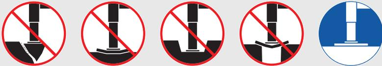
Verify that the extra support plates do not bend or sink into the ground.
