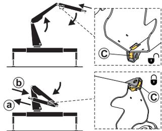
6. Lower the 1st boom completely (4) to the parking support of the base.
