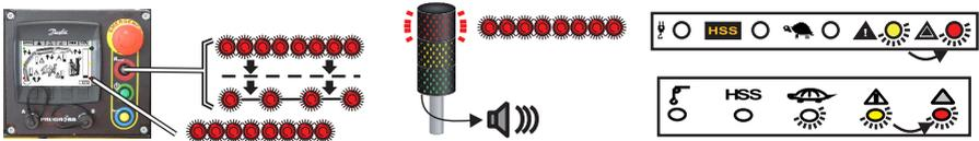
3. After a 10-second interval, the red lamp and the RESET button LED blink for 30 seconds (the waiting time).
