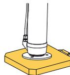
The maximum permitted ground inclination under the stabiliser leg plate is 5°.
