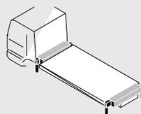
Common storage position with hydraulically tiltable stabiliser legs.
