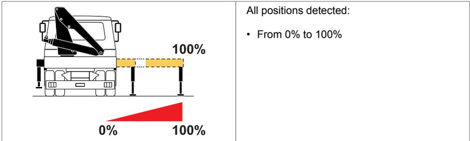
The position of the **auxiliary stabiliser extensions** is not detected proportionally by Progress to calculate the stability.
