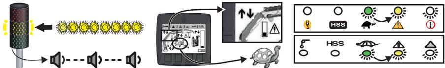
**When 100% of the maximum permitted pressure is reached, the system stops all functions that increase the pressure.**
