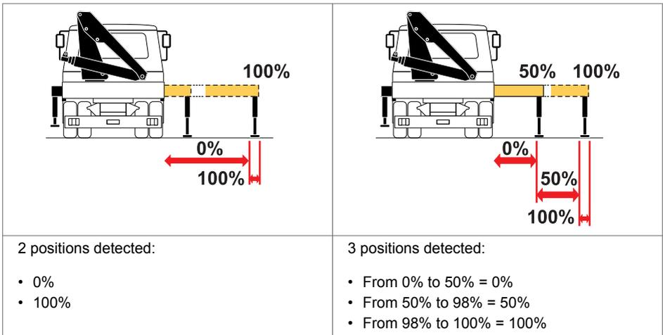
The complete crane operating area is subdivided into four sectors and their width varies according to the extension of the stabiliser extensions. Progress manages
