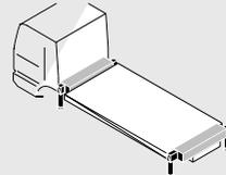
Common storage position with hydraulically tiltable stabiliser legs.
