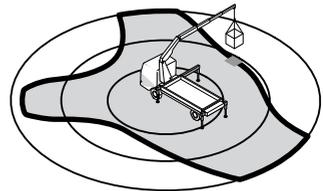
The position of both, **crane stabiliser extensions** and **auxiliary stabiliser extensions**, are detected proportionally by Progress to calculate the stability.
