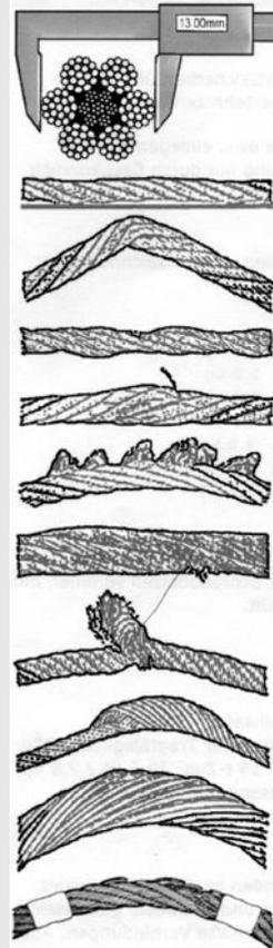
A rope has to be discarded, when there are number of ruptures in the outer layers according to DIN 15020; ISO 4309:
