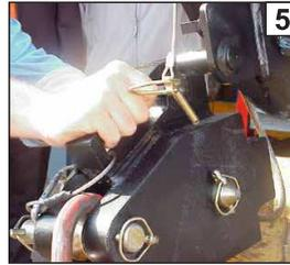
10. Rotate the counterweight carefully by 90° with the help of the appropriate handle.
