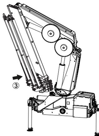
4. **Cranes with S-boom:** Start to lower the 1st boom until the 2nd boom is horizontal. Extend the extensions until the catcher (4) drops. Retract the extensions carefully to give the required parking width and the catch secures the boom. Continue to lower the boom system onto the parking support.
