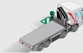
1. If the stabiliser system is manually controlled, push button
