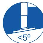
The maximum permitted ground inclination under the stabiliser leg plate is 5°.
