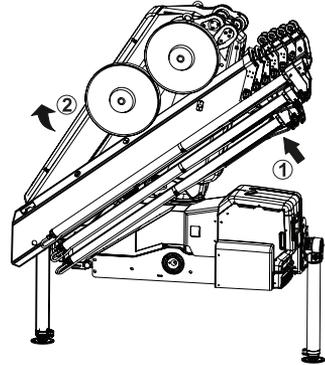
3. As soon as the 1st boom is raised to an angle where the 2nd boom can go free from the crane base, raise the 2nd boom (3).
