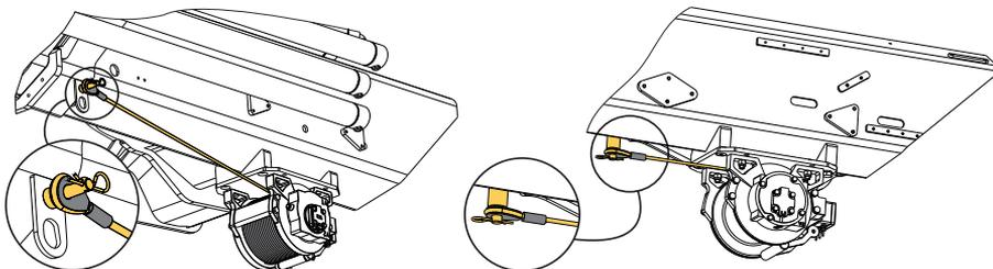
5. Remove the intermediate pulleys (if needed).
