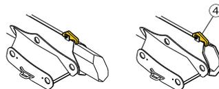
5. Lower the 1st boom until it is secured on the parking support (5).
