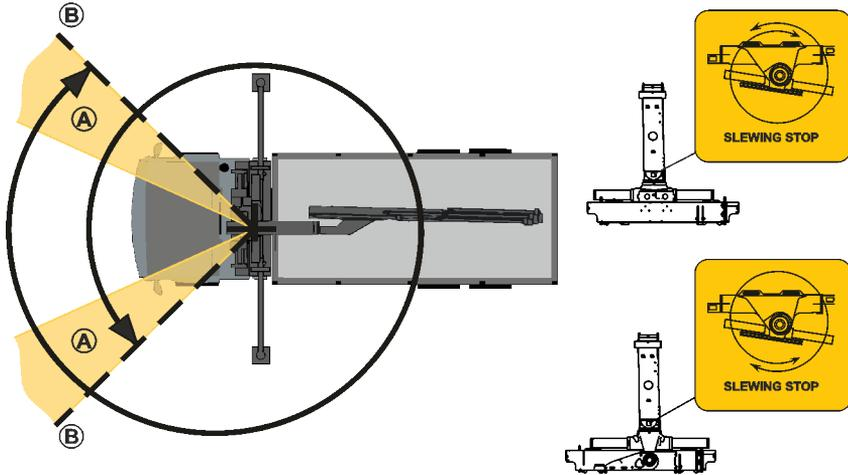
2. Slew the crane slowly in each direction to the slewing stop (B).
