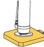
**The maximum permitted ground inclination under the stabiliser leg plate is 5°.**
