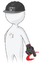
**Stop all crane movements / Hold the load in position**
