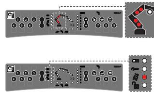
**Stabiliser system OLP:** No indication on the controller. See indications on the User Interface.
