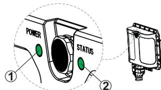
The LED is steady green = the gateway is operational and all connections are correct.
