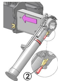
6. Lock the stabiliser leg lock (2) in the hole (3).
