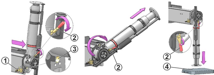
7. Put the extra support plate (4) onto the ground (if necessary).
