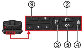
In each of the primary VIEWS, you can select different sub-VIEWS by pushing the same VIEW button repeatedly. The number of sub-VIEWS depends on the configuration of the crane.
