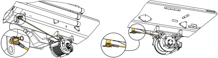
5. Remove the intermediate pulleys (if needed).
