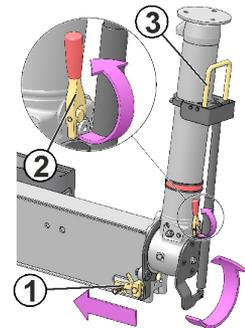
8. Retract the stabiliser extension completely. Follow the procedure: "Retract the stabiliser extensions".
