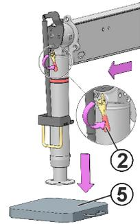
5. Extend the stabiliser extension. For manual stabiliser extensions, lock the extension.
