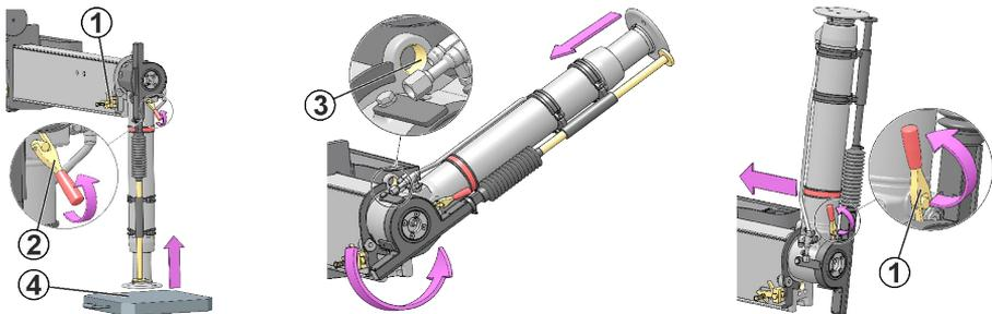
7. Retract the stabiliser extension completely. Follow the procedure: "Retract the stabiliser extensions".
