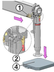
6. Put the extra support plate (4) onto the ground (if necessary).
