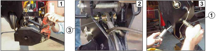
7. Unlock and disassemble the pin (2) on the counterweight [4].
