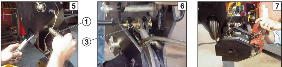
13. Fasten the hook to the counterweight with the fixing chain [7].
