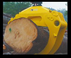
The heavy TX86B and the TX811B, with its wider jaws, can be installed on industrial cranes and excavators.
